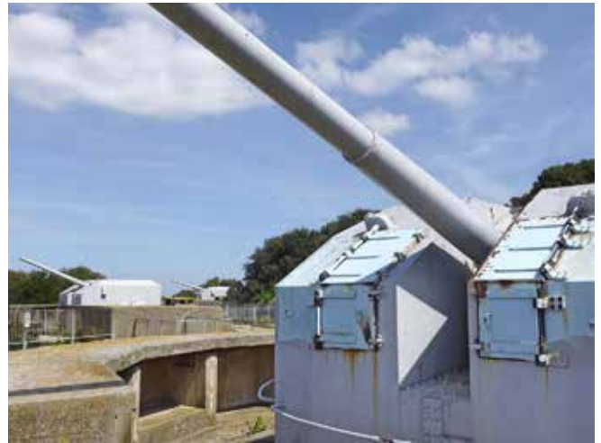
Princess Anne's Battery: three of the four 5.25-inch QF guns. The Mk1B turret mountings reflect their coast defence role
